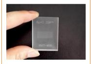
Standard Roughness Calibration Block Multi-engraved lines (Square Wave)
